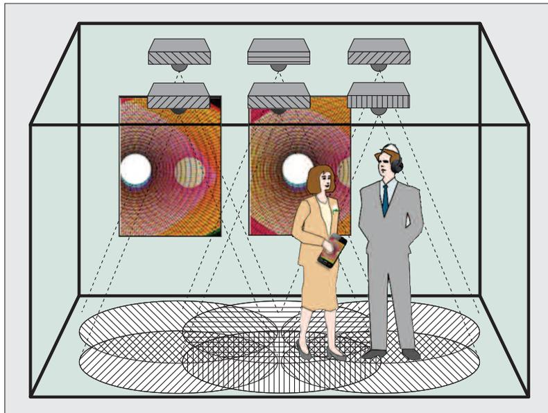
**Figure 1.** Two uses of visible light positioning in an art gallery. The headset worn by the man detects its position and plays recorded information relevant to the picture in front of him. The woman is using a location-aware service on her tablet computer.
