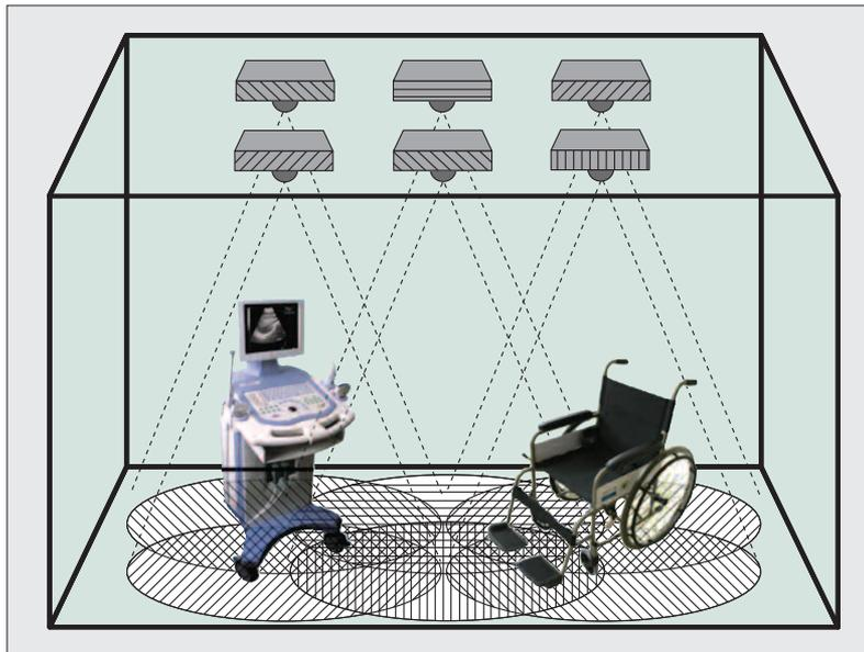
**Figure 2.** Use of visible light positioning for asset tracking in a hospital to locate the positions of the trolley and the wheelchair.
